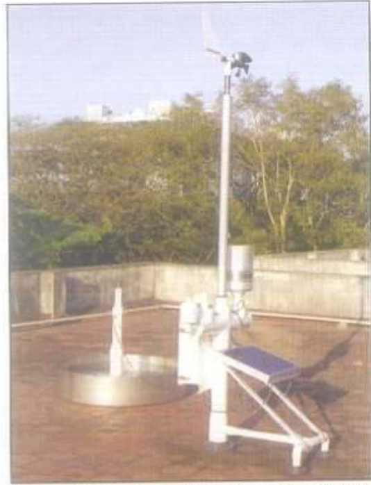
Automated Solar Powered Weather Station (NEERI)
